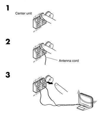
Turn the loop antenna until you have the best reception during AM (MW) broadcast program reception.
